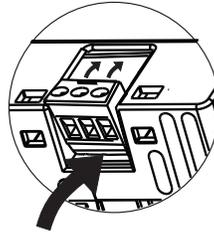
2. Gently push the top of the terminal block to rotate it into place.
