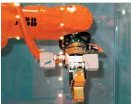
Robot arm equipped with wireless proximity switch
