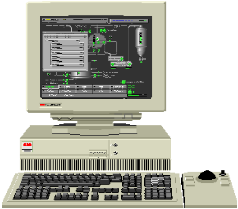
Figure 3-64. Advant Station 520 & 530 Configuration
