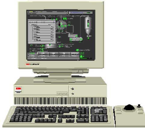
Figure 1-5. Advant Operator Workplace
