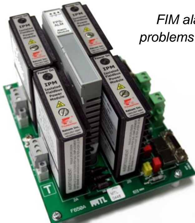
MTL-Relcom F650A Redundant Fieldbus Power System (DIN-rails included but not shown)
