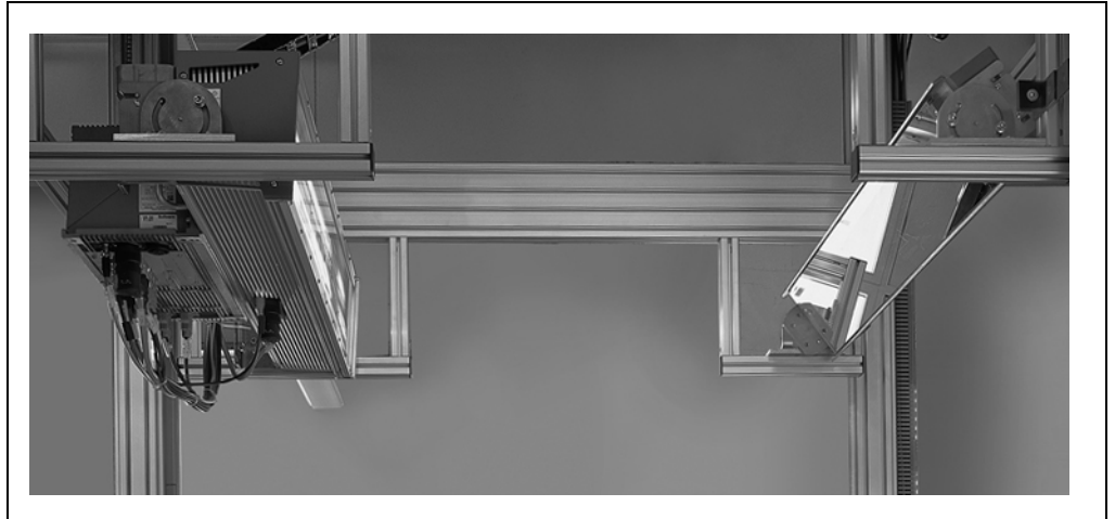
Fig. 3-7: ICR880/890 Camera System with deflection mirror for reading from above
