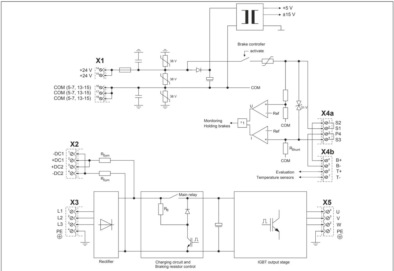
Figure 7: ACOPOS 1022, 1045, 1090 - Input/Output circuit diagram
