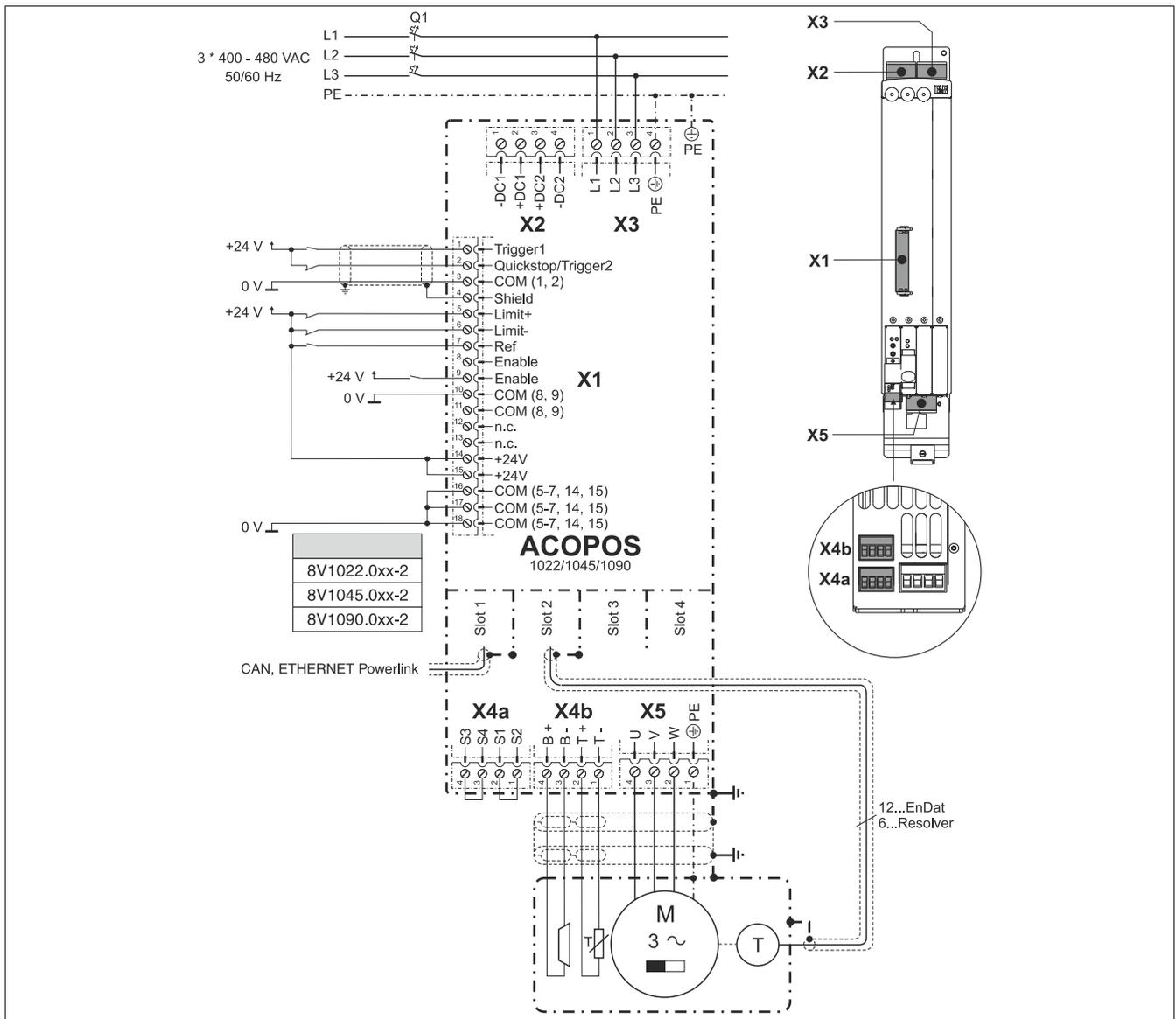
Figure 3: ACOPOS 1022, 1045, 1090 - Pinout overview
