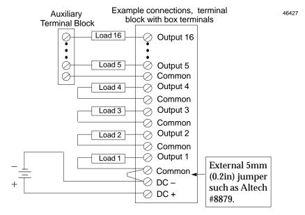
For an I/O Terminal Block with Barrier Terminals or an I/O Terminal Block with Wire to Board Connectors, an Auxiliary Terminal Block with Barrier Terminals might be connected as shown in the following example.
