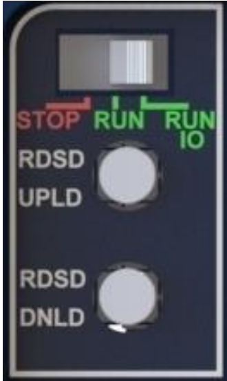
Figure 11: CPE330 RUN/STOP Switch and RDSD Switches
