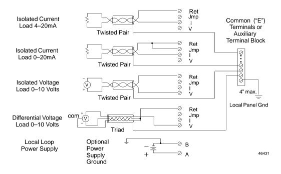
Instrumentation grade shielded twisted pair or 3 wire twisted (triad) wire should be used for best noise immunity. The shield should be terminated at a local panel ground near the module.
